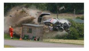
Following a massive accident that saw a Ginetta G50 explode into a fireball when the remote filler hoses were severed, ATL reacted to prevent any such incident ever occurring again.
